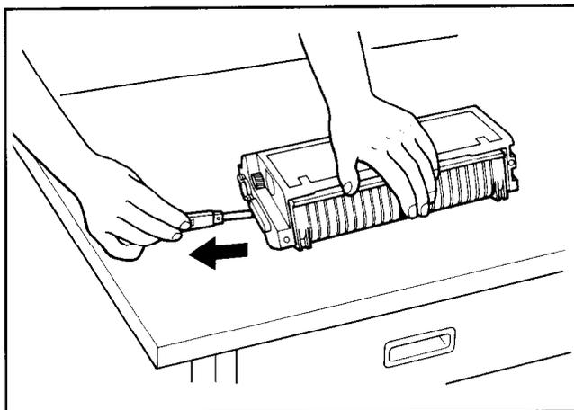
Make sure that the tab is pulled smoothly in a direction parallel to the flat surface. Otherwise, the tape may break or snap, making the cartridge unusable.
