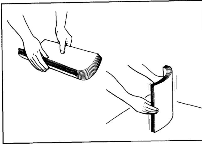
5. Align the right side of the stack of paper with the right-hand paper guide. Slide the paper stack gently into the printer as far as it will go. Make sure that the height of the paper stack does not exceed the mark on the paper guide.
