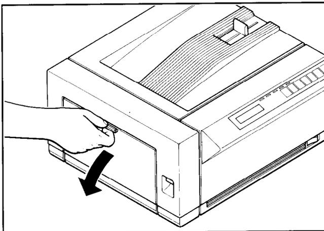
2. Hold the arrow at the center of the multi-purpose tray, then pull out the extension tray.
