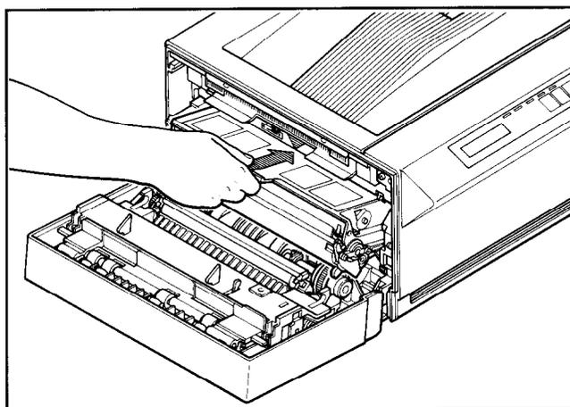
7. Slide the cartridge into the printer gently.
