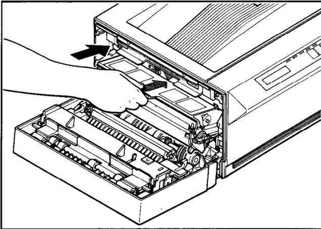
If vertical white streaks still appear after the toner inside the cartridge has been re-distributed, the cartridge needs to be replaced. See “2.2 Installing the EP-L cartridge” for replacing the cartridge.
