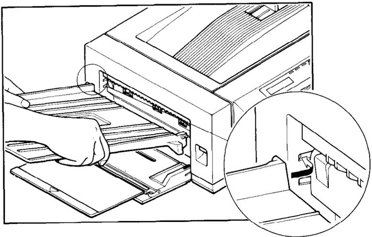
When face-up printing is finished and the multi-purpose tray is closed, the printer automatically switches back to face-down delivery.
