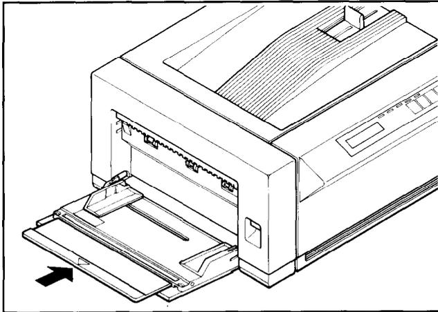
2) If the face-up tray is installed, remove it.
