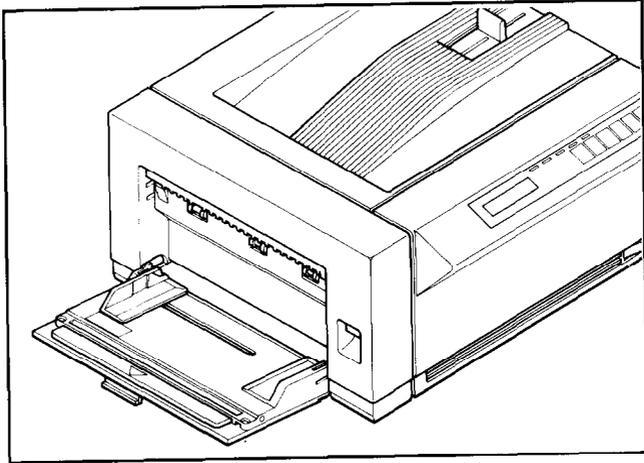
3. Press the release button (at the right ) upwards and open the cover.
