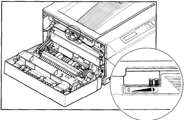
**NOTE:** The density adjustment lever has four settings from left to right. As you move the lever, it clicks at each of the two positions in the middle.
