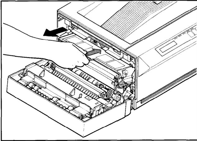
**NOTE:** If it is difficult to remove the EP-L cartridge, press the green lever located at the right, and try again.
