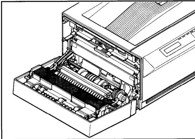
Although the printer's cover is closed while printing, it will need to be opened when replacing the EP-L cartridge when clearing paper jams. Open or close the cover in the following way:
