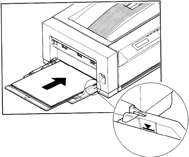
6. Slide the left-hand paper guide so that it touches the left side of the paper stack. Make sure that the paper guide does not press too tightly or fit too loosely against the paper stack. Otherwise, this can cause paper jams or other problems.
