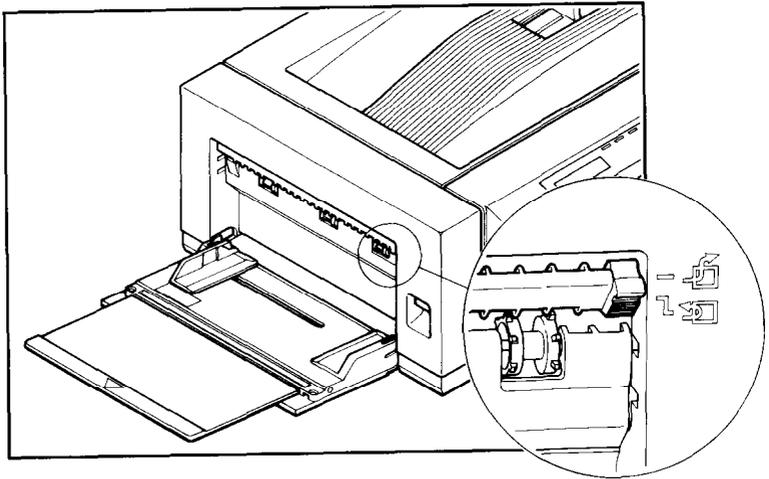
3. Attach the face-up print tray to the side cover of the printer. Fit the pegs at the sides of the tray into the holes in the printer.
