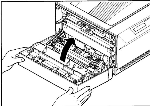
2. Lift the multi-purpose tray and close it until it latches on both sides.
