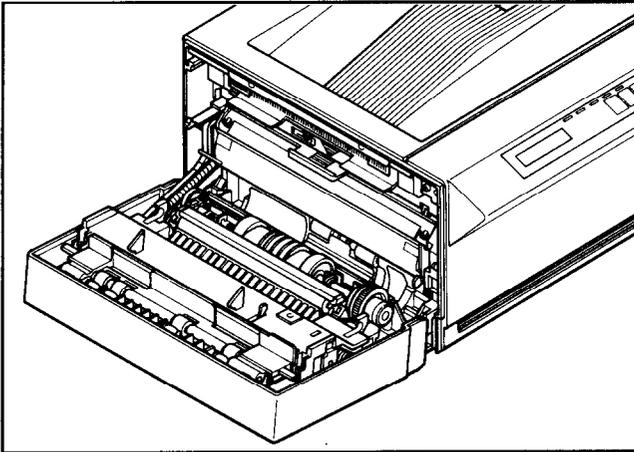
**NOTE:** Remove the two orange stoppers by pushing the lower part of the stoppers upwards and removing it (as shown in the illustration below).
