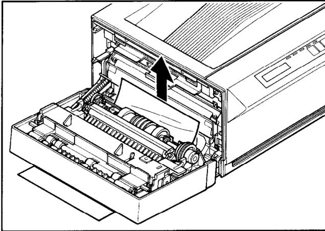
**CAUTION:** The fixing assembly area becomes extremely hot when the printer has been operated for some time. Never touch this area when the printer is open. Otherwise, personal injury may result.
