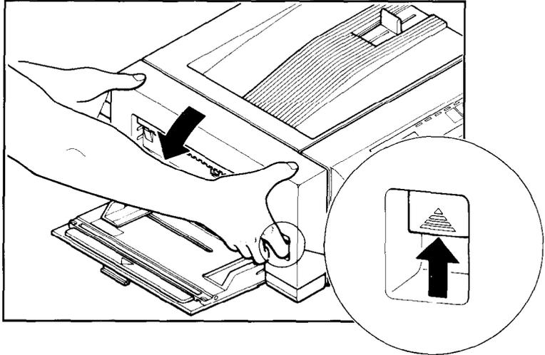
3. To increase print density, move the density adjustment lever to the right. To reduce the density, move the lever to the left.
