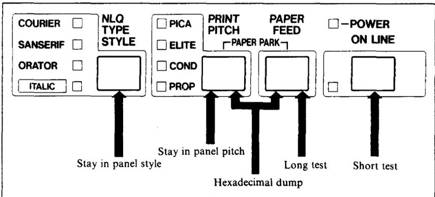
Figure 2-4. Power-up functions of control panel
