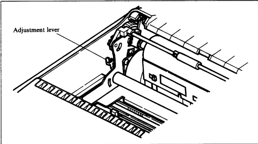
**Figure 1-14.** Adjusting for different thicknesses of paper
