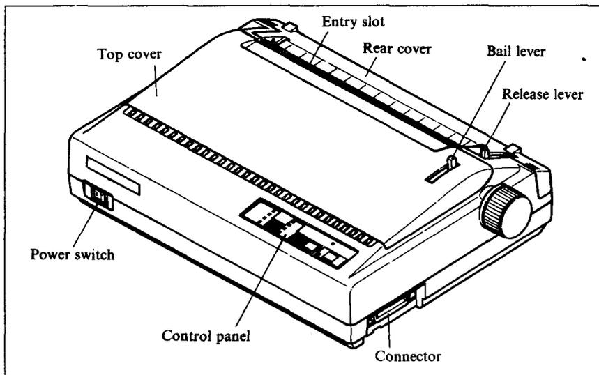
**Figure 1-2.** The printer's external parts
