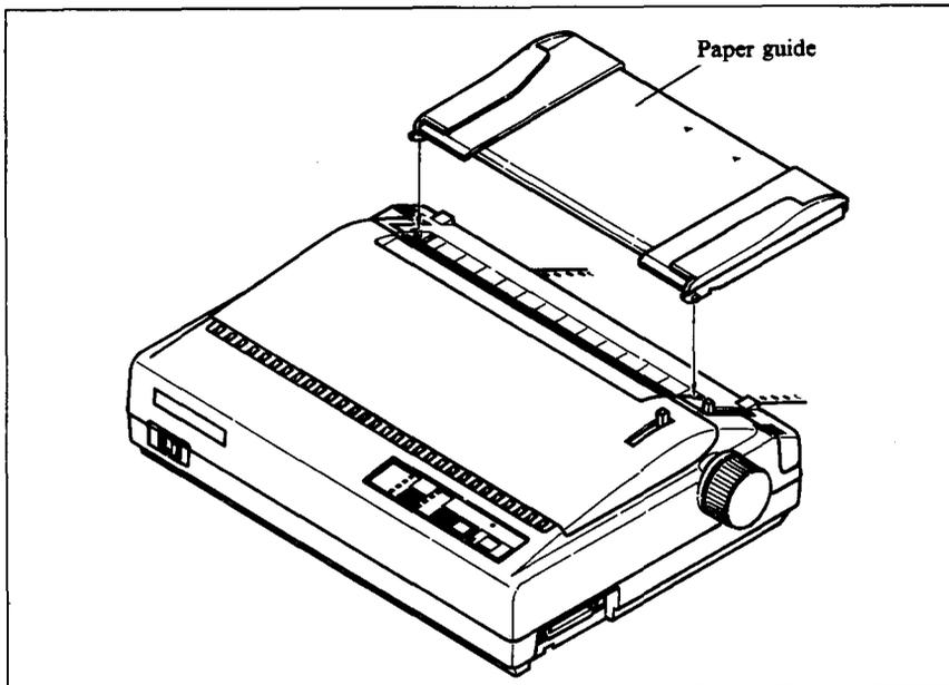
**Figure 1-12.** Mounting the paper guide for fanfold forms
