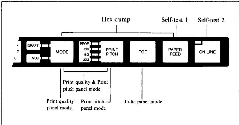
**Figure 2-3.** Extra functions while turning on the printer.
