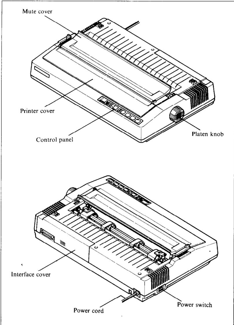
**Figure 2-1.** Front and rear views of the printer.
