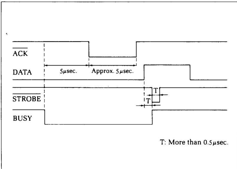
Figure F-1. The interface timing diagram.
