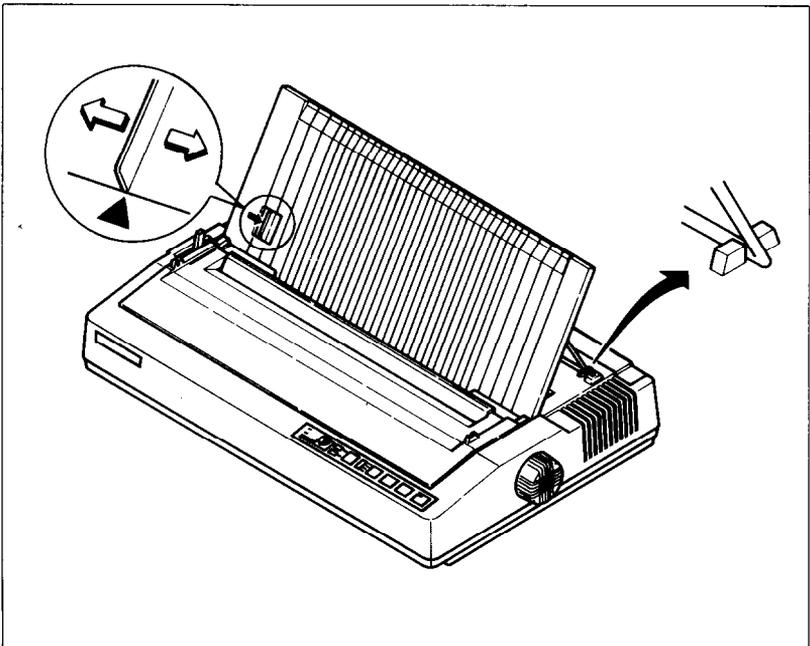
**Figure 2-7.** Prop up the paper guide by inserting the guide stand in the notches provided for it.
