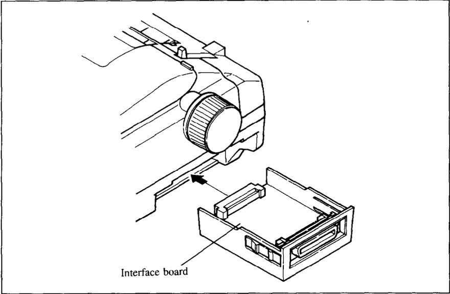
**Figure 1-9.** Replacing the interface board
