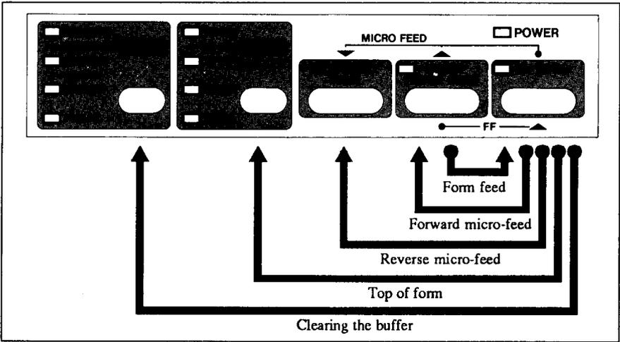
Figure 2-6. Switch combination functions of control panel
