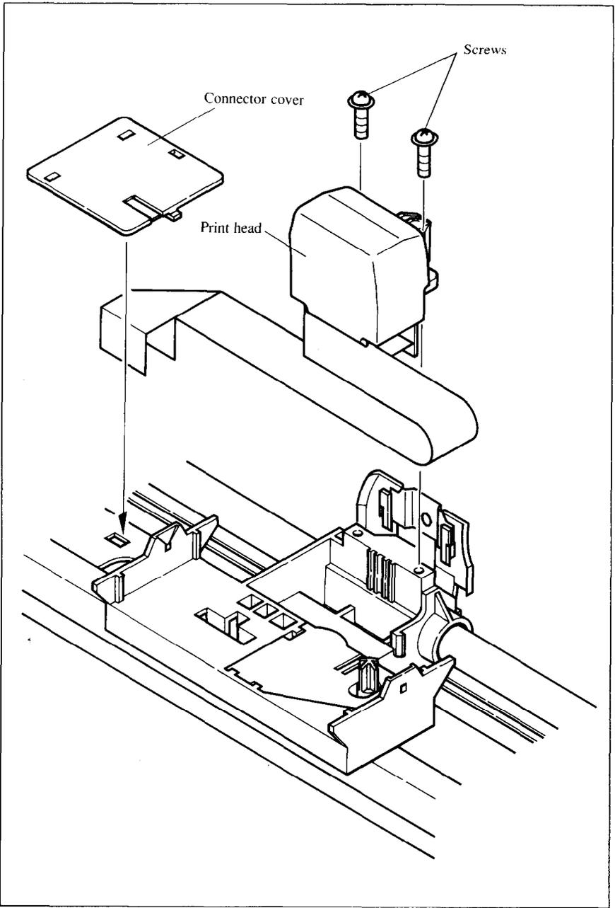
**Figure 7-4.** Replacing the print head
