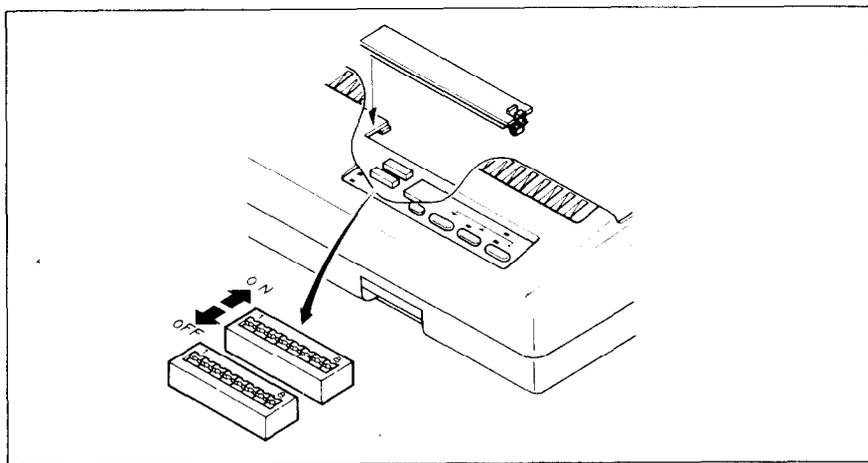
**Figure 3-1.** DIP switches
