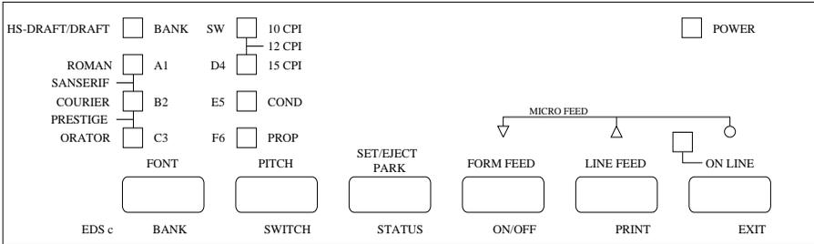
This chapter describes control panel functions that can be performed while the printer is turned on and either on-line or off-line. The buttons perform different functions in the EDS and Dot Adjustment Modes. Functions of control panel buttons in these modes are described in the relevant sections covering them.
