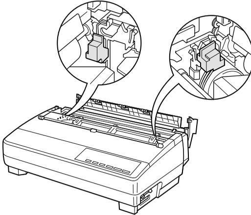
A piece of cardboard is inserted into the printer to protect components during shipping. Be sure to remove it before using the printer.
