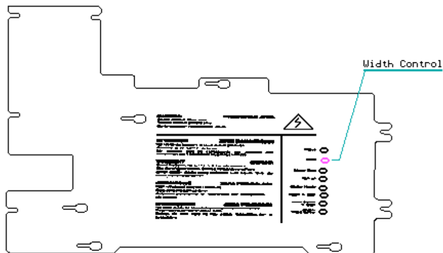
Figure 8-22. Adjusting the CRT Width Control
