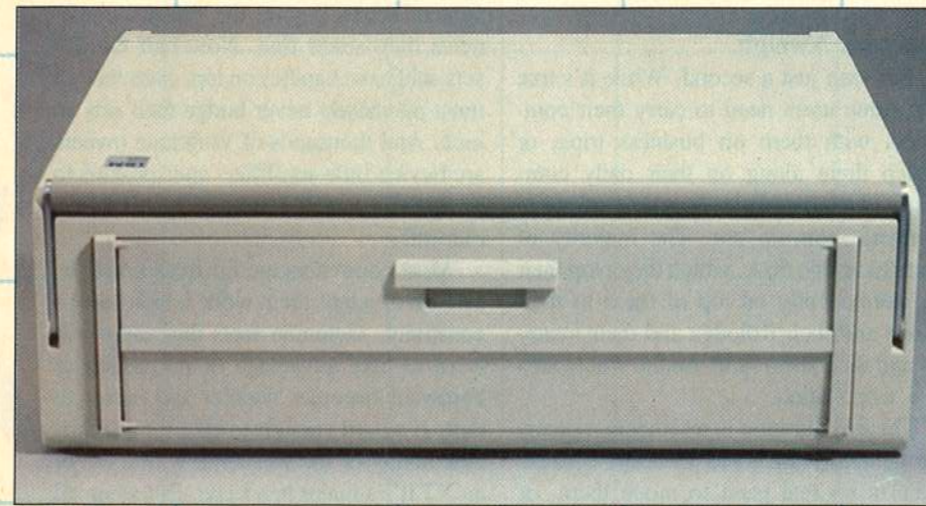
Spring tension holds rear door closed for travel.
