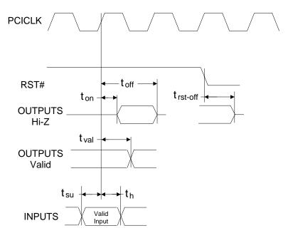
Figure 2. PCI Timing Measurement Conditions
