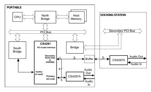
Figure 6. Portable Docking Station Scenario
