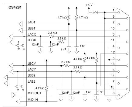
Figure 12. Joystick Logic
