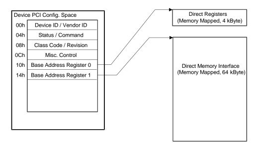
Figure 8. Host Interface Base Address Registers
