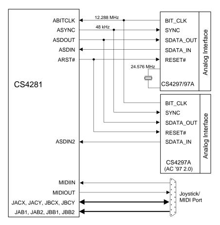
Figure 10. Dual AC '97 Codec Connection Diagram
