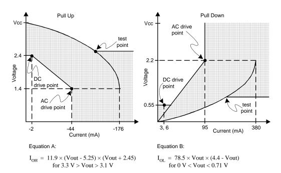
Figure 1. AC Characteristics
